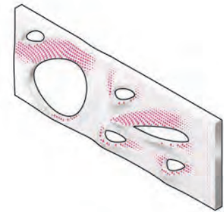
Apply glassing, resin and graphics After applying a first coat of fiberglass and resin the panel is sanded and applied graphics. A final gross coat seals and finishes the panel
