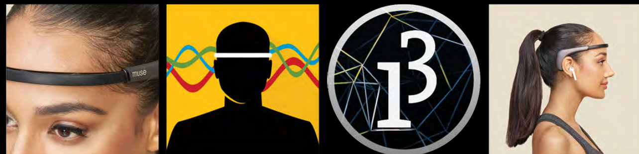
Muse Headband: Brain Wave Data recorded: Alpha, Beta, Theta, Gamma, Delta Mind Monitor: Open API App by James Clutterbuck: Allows for real time streaming from your Muse Device Processing: Coding software by Ben Fry & Casey Reas: Tool used to develop visual and audio manipulations Output: Sound and Visuals: Output gets then delivered in real time back to the user through both visual and auditory representations.
