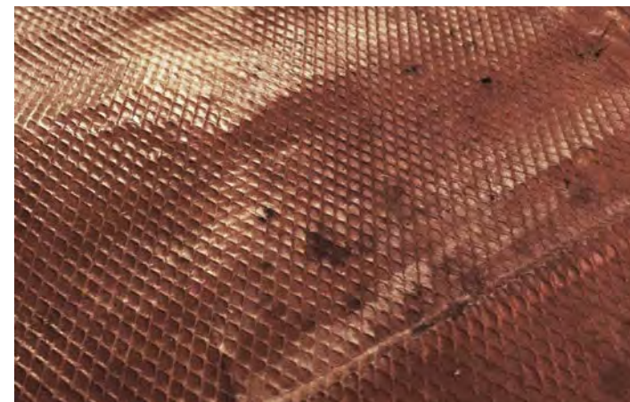
5) Close up of Image 4: Two pieces of culture combined with metal mesh integrated in the middle. Culture fuses together when still wet and in contact.
