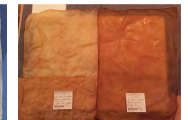
Process images of each stage of the cellulose: fermentation with mother culture - extract top film of cellulose and wash - place on surface or hang for drying (we altered this process when starting to insert different materials and substances into the fermentation and drying process)
