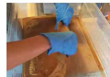
Process images of each stage of the cellulose: fermentation with mother culture - extract top film of cellulose and wash - place on surface or hang for drying (we altered this process when starting to insert different materials and substances into the fermentation and drying process)
