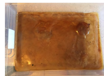
Process images of each stage of the cellulose: fermentation with mother culture - extract top film of cellulose and wash - place on surface or hang for drying (we altered this process when starting to insert different materials and substances into the fermentation and drying process)
